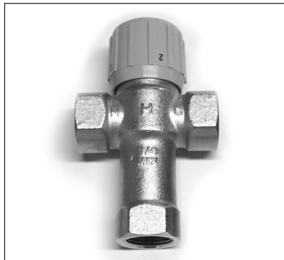
Figure 24 - Adjust Thermostatic Mixing Valves at each point-of-use to 120°F/49°C or lower.
