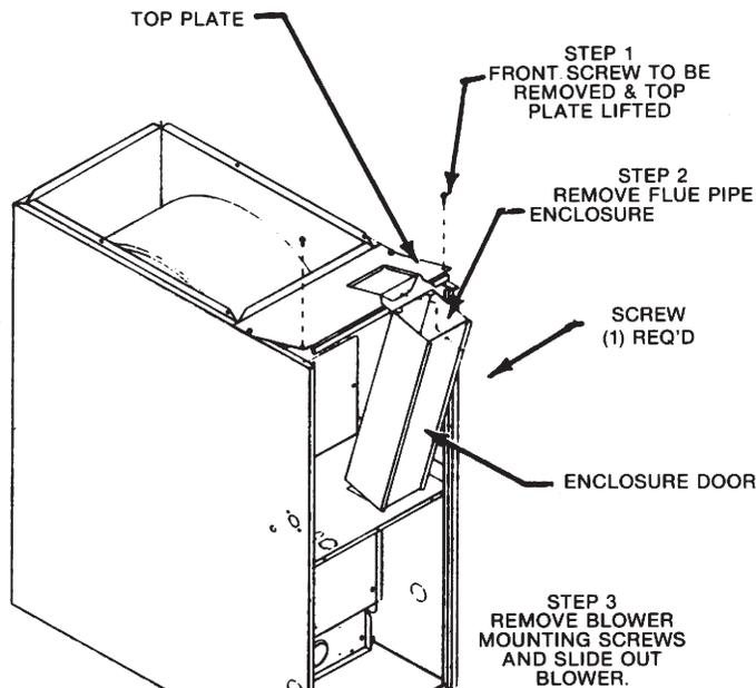
NOTE: FLUE PIPE ENCLOSURE & ENCLOSURE DOOR MUST BE REMOVED FOR BLOWER REMOVAL.
