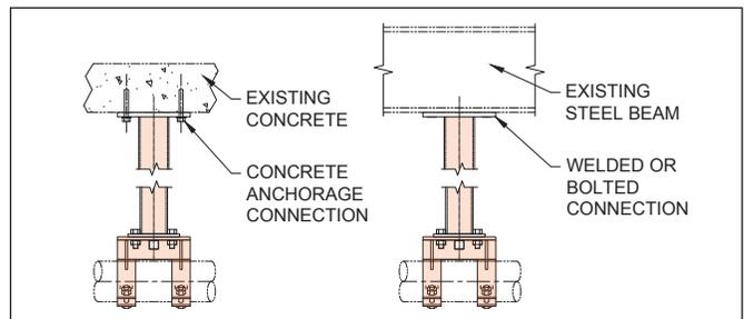
FIGURE 1.2 TYPICAL INSTALLATION OF PRODUCT A81/A82/A83 TO CONCRETE AND STEEL STRUCTURE
