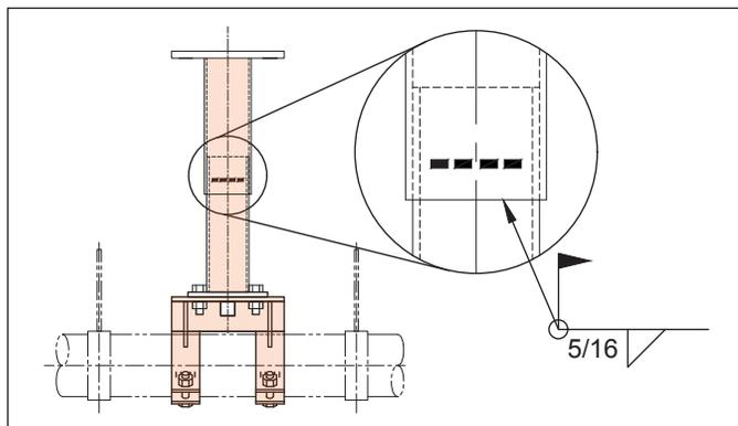
FIGURE 3. A81 AND A82 ADJUSTABLE STRUT INSTALLATION
