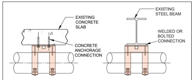
FIGURE 1.1 TYPICAL INSTALLATION OF PRODUCT A84 TO CONCRETE AND STEEL STRUCTURE
