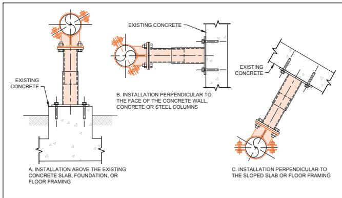
FIGURE 5. ALTERNATE INSTALLATION ORIENTATIONS FOR A81, A82, AND A83 PRODUCTS
