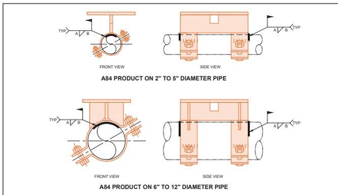
FIGURE 6. WELDING DETAILS FOR ENHANCED A84 CAPACITY
