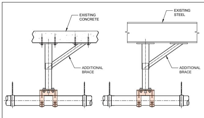
FIGURE 2. TYPICAL INTERMEDIATE STEEL FRAME CONNECTING PRODUCT A84 TO SUPPORTING STRUCTURE
