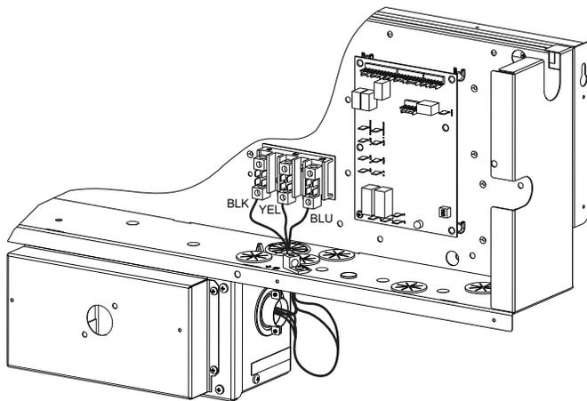
**Fig. 28 — Location of Non-Fused Disconnect Enclosure**
