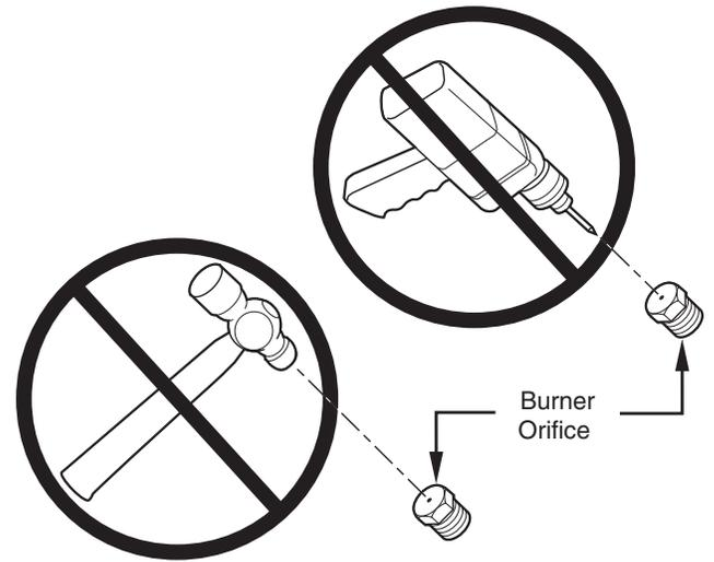
**Fig. 23 — Orifice Hole**
