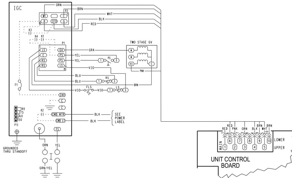
**Fig. 44 — Typical IGC Control Wiring Diagram**
