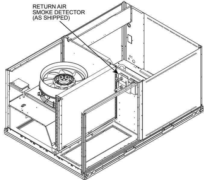
**Fig. 51 — Return Air Smoke Detector; Shipping Position**
