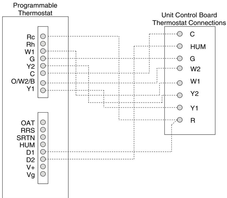
**Fig. 37 — Typical RGV090-150 Unit with Hot Gas Re-Heat Dehumidification System and Edge® Pro Thermidistat Device**
