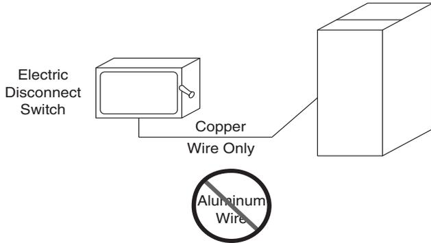
**Fig. 27 — Disconnect Switch and Unit**
