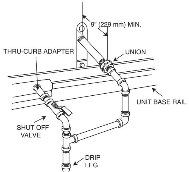
**Fig. 20 — Gas Piping, Typical Curb Sidewall Piping (Example 1)**
