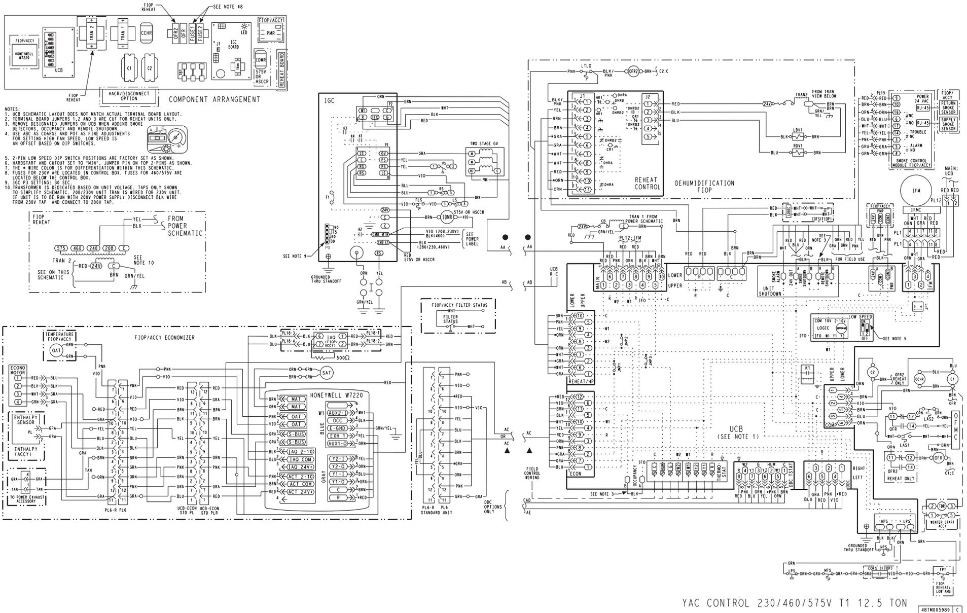
Fig. 40 — Typical Control Wiring Diagram, Electro-Mechanical with W7220 – RGV150, 230/460/575-3-60 Units Shown
