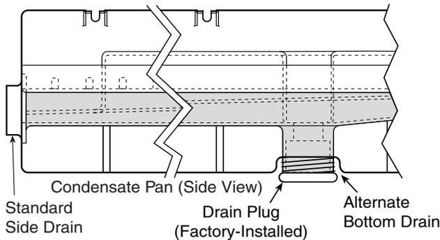
**Fig. 24 — Condensate Drain Pan (Side View)**
