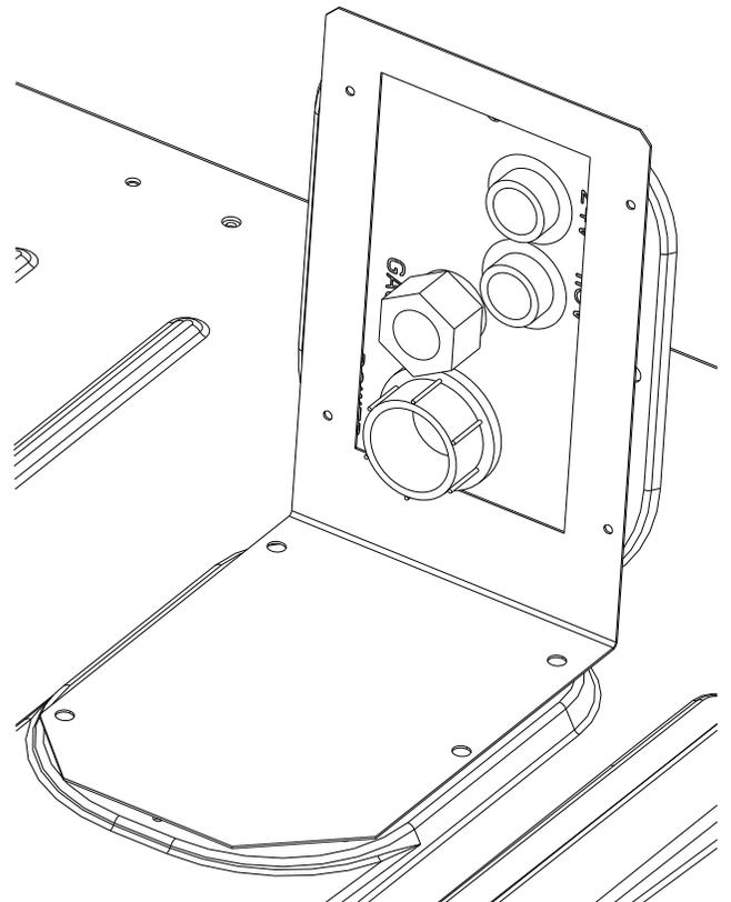
**Fig. 17 — Thru-the-Base Fitting Assembly (Shown in Shipping Position)**
