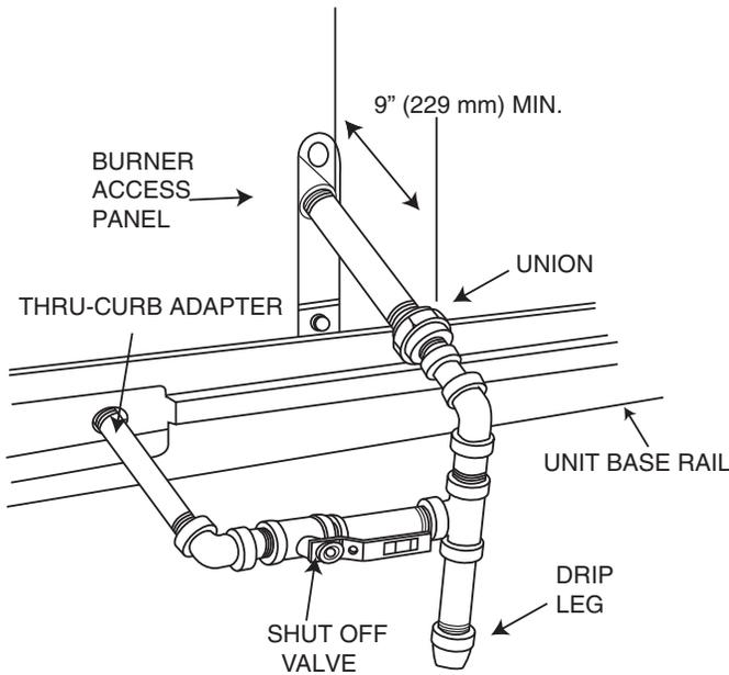
**Fig. 21 — Gas Piping, Typical Curb Sidewall Piping (Example 2)**
