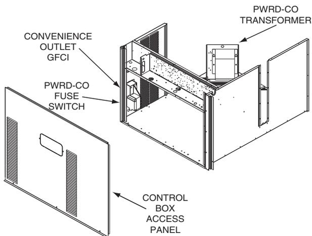
**Fig. 30 — Convenience Outlet Location Installing Weatherproof Cover**
