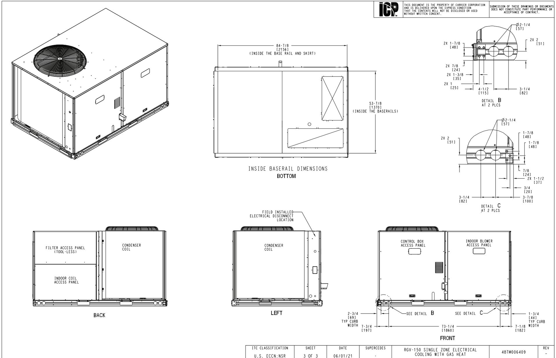
Fig. 3 — Unit Dimensional Drawing – Size 150 (cont)
