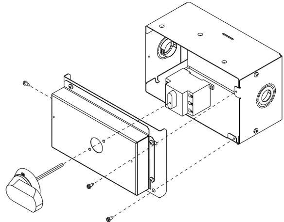
**Fig. 29 — Handle and Shaft Assembly for NFD**
