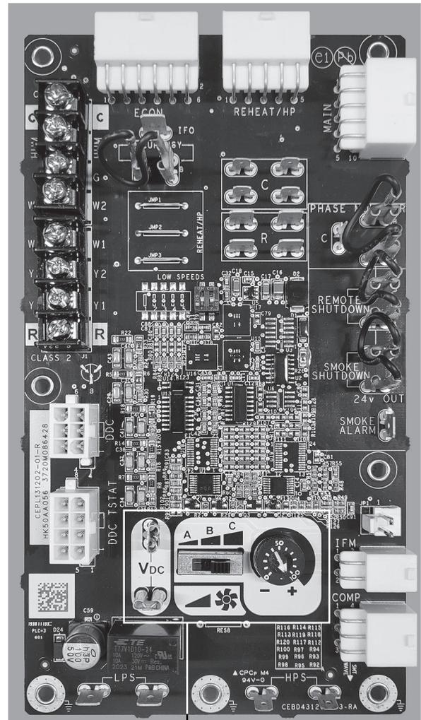
Fig. 53 — UCB Fan Speed Controls
