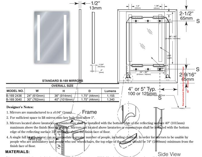
Glass — 0.19" (5mm) thick safety mirror with 0.14mm PVC film backer with frosted sandblasting/Wall Hanger Extruded Back — Aluminum channel with mounting holes.
