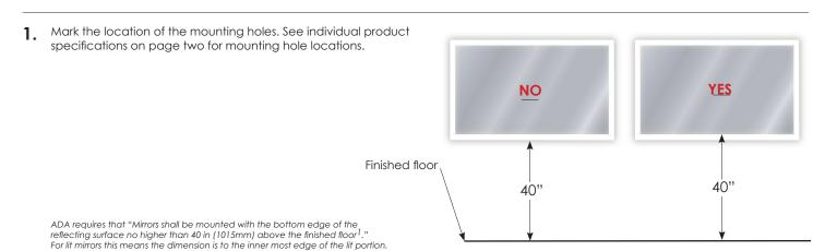
2. Install included #14 round slotted wood mounting screws into pre-marked holes. Note, all mirrors must be installed in contractor supplied blocking.
