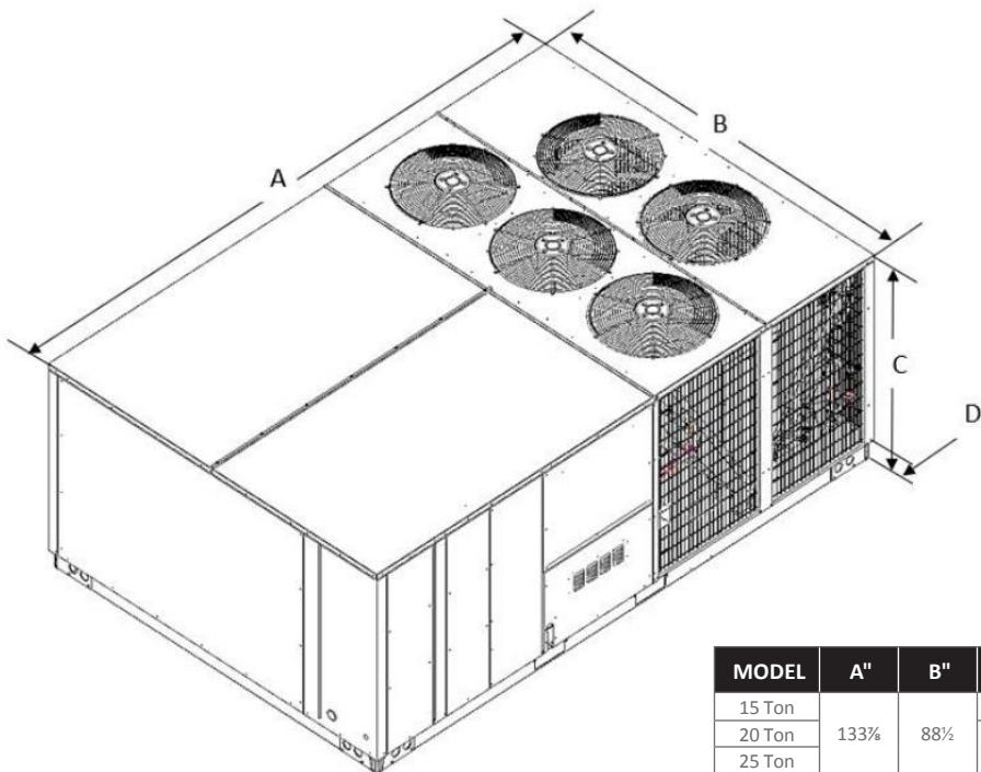
**NOTE:** 15 ton has 3 fans; 20 ton has 4 fans; 25 ton has 5 fans
