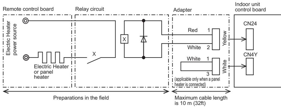
◆For relay X use the specifications given below Operation coil
