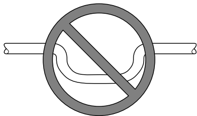
Fig. 17 – Recommended Condensate Trap
