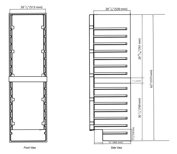
EdgeStar, 8606 Wall St, Suite 1600, Austin, TX 78754 www.edgestar.com • contact@edgestar.com **EDGESTAR**<sup>®</sup> Document Type: Dimensional Drawing Model: CWR1552DD Version: 2.0 12092019
