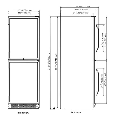
EdgeStar, 8606 Wall St, Suite 1600, Austin, TX 78754 www.edgestar.com • contact@edgestar.com **Exterior Dimensions**
