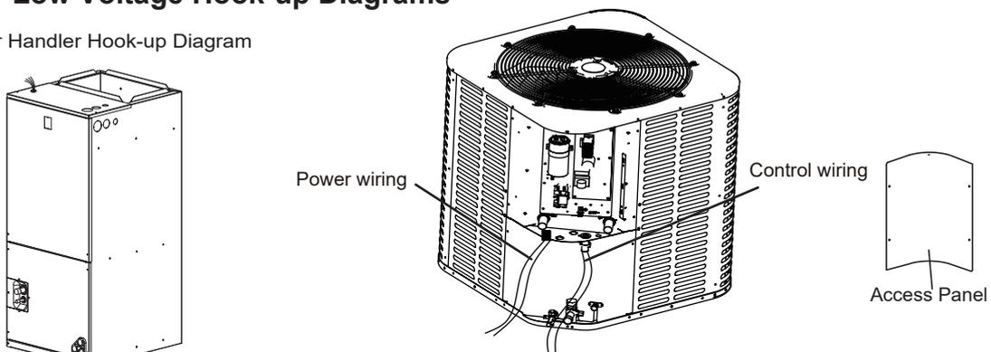
Low Voltage connection must be made inside the outdoor unit case.
