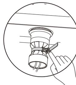
2. After installation or maintenance, the tightening belt shall be tightened, can not be loosened or discarded; the control box access panel must be installed and the screws must be tightened.
