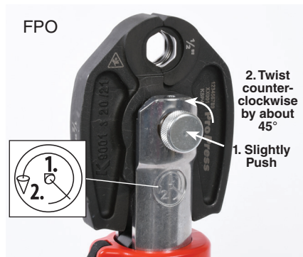
Figure 7 – Opening The Attachment Mounting Pin
