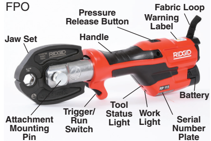
Figure 1 – RIDGID RP 115 Press Tool with Jaw
