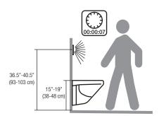
Installing highly reflective surfaces (such as mirrors) in the immediate vicinity of the water closet flush control should be avoided, as these can lead to incorrect releases and malfunctions.
