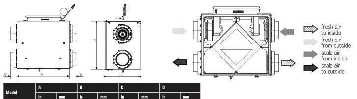
ATMO 200H 23  $7_{8}$  606 29  $1_{2}$  751 16  $5_{8}$  423 21  $7_{16}$  546 Clearance of 22" (559 mm) in front of the unit is recommended for removal of core. All units feature three foot plug-in power cord with 3-prong plug.
