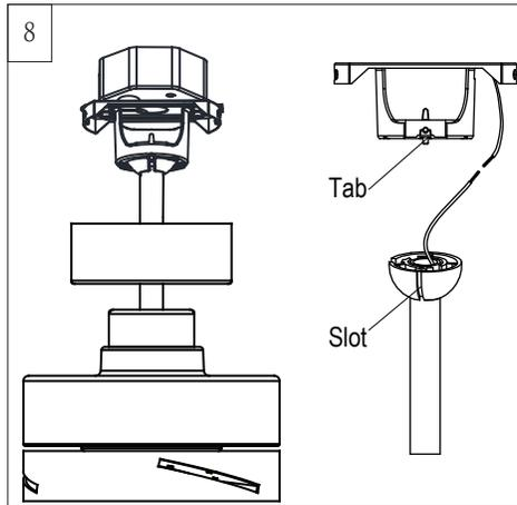
Install ball end of downrod into mounting bracket opening. Align (engage) slot on ball with tab with tab on mounting bracket.
