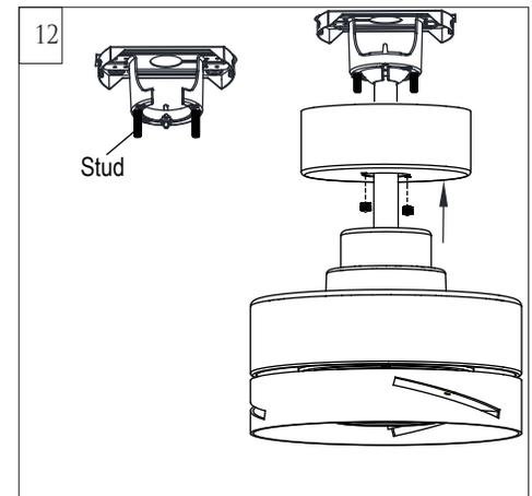
Lift Canopy allowing the 2 studs to protrude through the canopy and install the knurled nuts as shown. Tighten the knurled nuts securely. The canopy should adjust for any irregularity in the ceiling or Outlet box.
