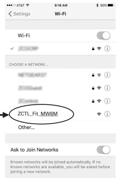
Select the Fit's SSID → The last 4 digits (underlined) will match the first 4 digits of your Fit controller's Device ID.
