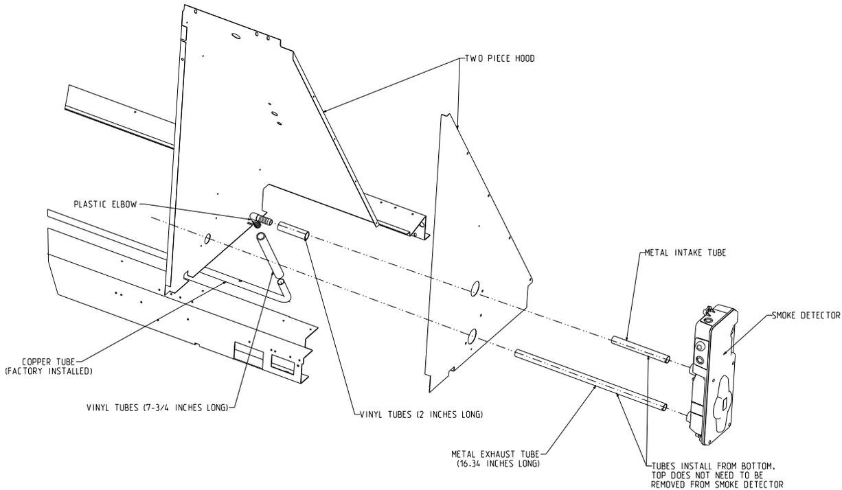
4. Slide one 2" piece of the vinyl tubing provided onto the short smoke detector inlet tube which protrudes out of the back side of the smoke detector. Push this piece of vinyl tubing onto the inlet tube until it contacts the end of the plastic extension on the backside of the smoke detector.
