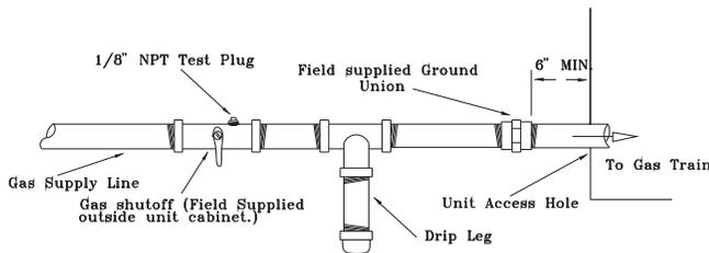
**Figure 20. Typical unit gas train configuration**
