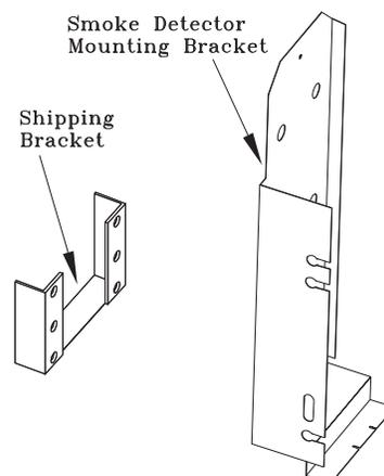
Figure 25. Return air smoke detector for downflow units
