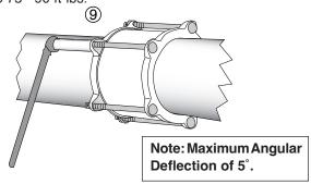
Wait 10 minutes and retighten to account for settling of the gasket.
