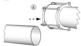
Note: Flexible Couplings do not provide protection against possible pullout of pipe ends in unrestrained conditions.
