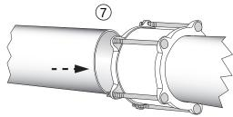
**Step 8** • Center coupling over pipe ends using the reference marks described in Step 4.
