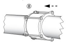
**Step 9** • Tighten bolts such that the end ring flanges remain parallel and the gaskets are evenly compressed. Bolt tightening should be done evenly, alternating to diametrically opposite positions at approximately 20 ft-lbs increments. Tighten to 75 - 90 ft-lbs.
