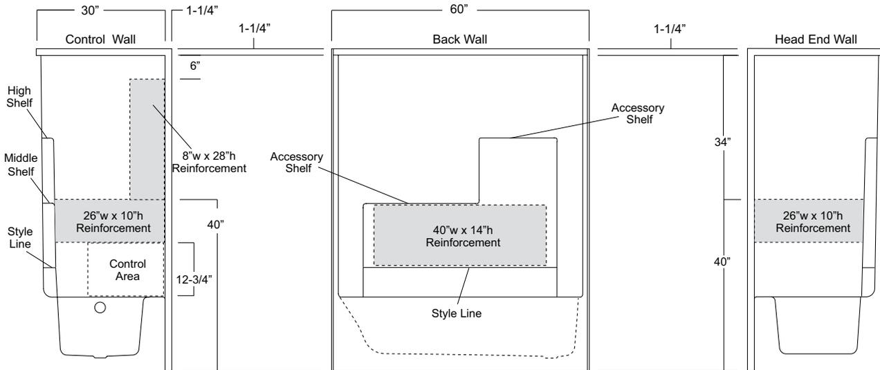
**Package Order No.: 3SM (3-side, mid-level wall reinforcement)**
