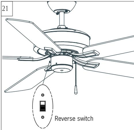
21 Setting the reverse switch in the down position will result in downward airflow and setting the switch in the up position will result in upward airflow.
