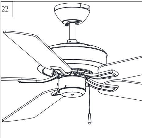
22 Install fan pull chains to preassembled pull chain on fan. Pull chain provided.
