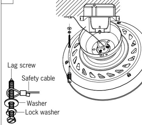
For Canadian installation and for USA fan and light kit combinations over 35 lbs, in both flush and downrod modes the safety cable must be installed into the house structure beams using 3" lag screws, washers and lock washers provided. Make sure that when the safety cable is fully extended the lead wires are longer than the cable and no stress is placed on the lead wires.
