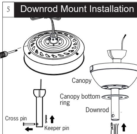
Partially loosen downrod set screws from yoke at top of motor assembly. Remove preassembled cross pin and keeper pin from downrod. Place downrod over canopy and canopy bottom ring. Thread lead wires and safety cable from motor assembly through downrod.
