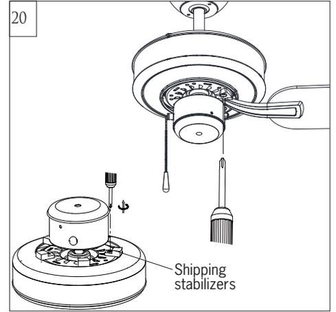
20 Remove shipping stabilizers from motor assembly. Install the blade assembly to motor using the preinstalled screws. Tighten screws securely. Repeat this process for remaining blade assemblies.
