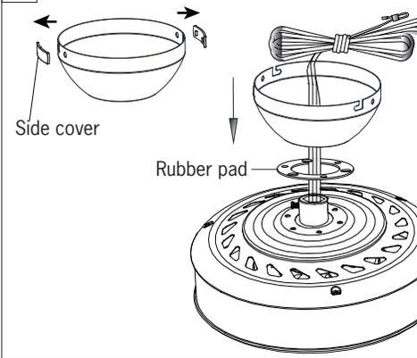
Remove side covers from canopy exposing 4 holes. 2 closed holes and 2 open "L" shape holes.
