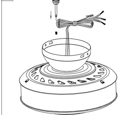
Reinstall the 3 set screws remove in step 12. Tighten screws securely.
