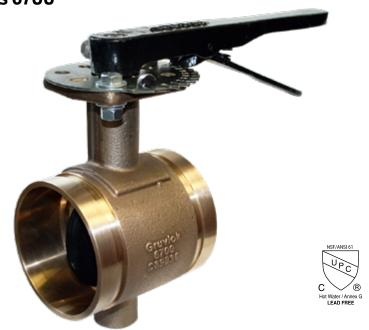
The lever handle bronze body butterfly valve is designed for use with grooved copper tubing (CTS), fittings and couplings. This valvefeatures a 10 position lever handle, bronze body and EPDM rubber encapsulated disc. Both bronze valve body and the EPDM rubber disc obtained certification to ANSI/NSF 61 for use in potable water systems and is rated to 300 PSI.
