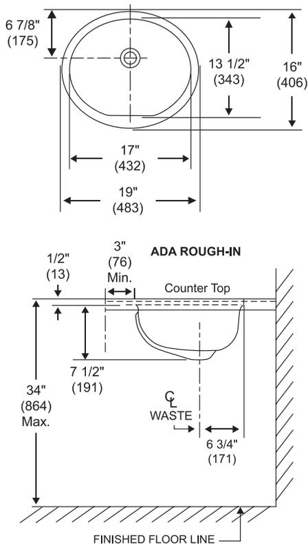
Dimensions may vary (+) or (-) 1/8". Dimensions shown in parentheses are in millimeters: 25.4 mm = 1 inch. Note: Fixture dimensions are nominal and conform with dimension and performance requirements of ASME/ANSI Standards A112.19.4M. Dimensions subject to change or cancellation without notice. Briggs is not responsible for the use of superseded or voided specification information.
